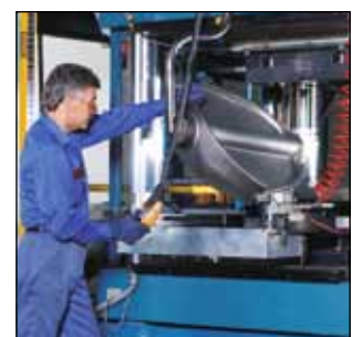
The rubber is vulcanised onto the wedge by AVK GUMMI A/S, one of Europe's leading manufacturers of high technology moulded rubber components.
