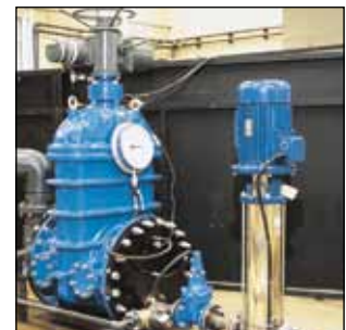
During laboratory tests at BHR Group in the UK the AVK PowerSaver™ valves have proved to be considerably less power consuming than gate valves of traditional design.
